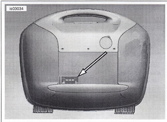
Figure 2. Left Side Case Reflector Mounting Location
