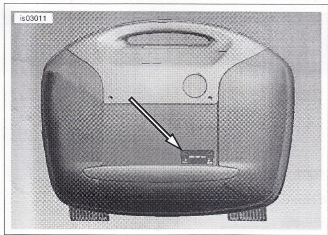
Figure 3. Right Side Case Reflector Mounting Location
