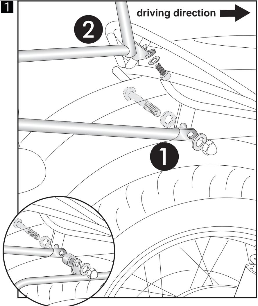
**Control all screw connections after the assembling for tightness!**
